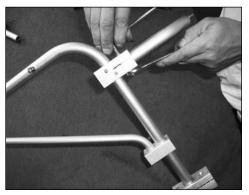
1.4 Hold the connector block screw steady with an open-end wrench while securing the clip connector screw with a hex wrench.
