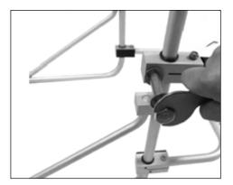
4.1 Use the big open-end wrench (I) to unscrew the wheel bolt from the right wheel connector found on the lower right arm assembly (A).
