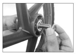
4.2 Insert a metal washer thru the bolt then insert thru the wheel hole. Insert another metal washer thru the bolt on the other side of the wheel.
