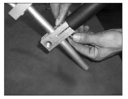
2.2 Place the connector block screw and the clip connector screw together inside the clip connector.
