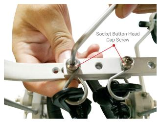
4.1. Loosen and remove Socket Button Head Cap Screws on the Front and Rear Harness Bars with the Hex Wrench.
