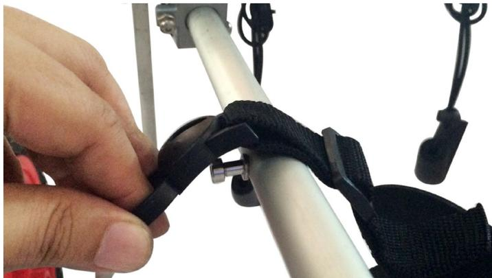
2.9. Fasten the plastic clamp to the side arm bolt
