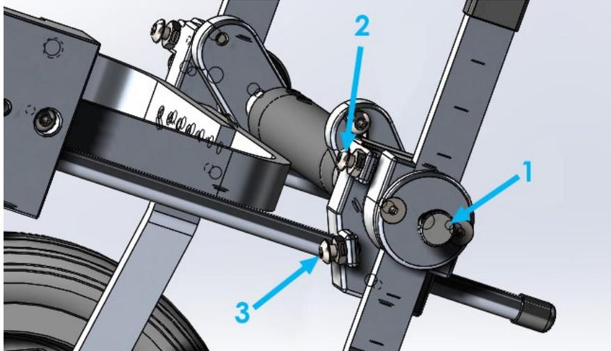
6.2. To release the SitGo function from its non-collapsible setting to the collapsible setting, loosen the number 3 screw indicated in the picture above until you are able to collapse the wheelchair all the way down.
