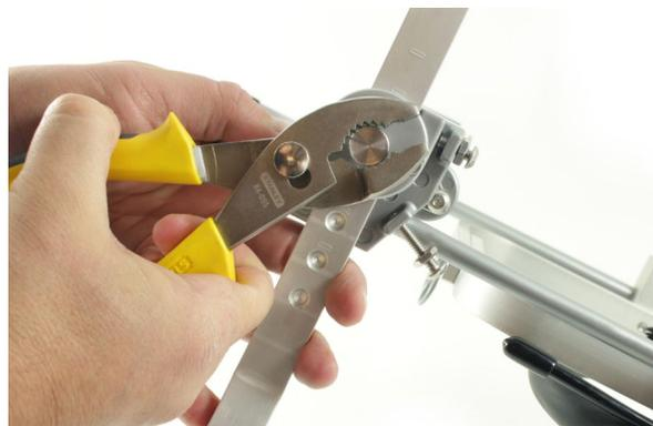
3.5. Adjust to desired height. Line up top of round wheelbar assembly to scored line like so to ensure that thumbscrew lines up into corresponding divot. Tighten with pliers.
