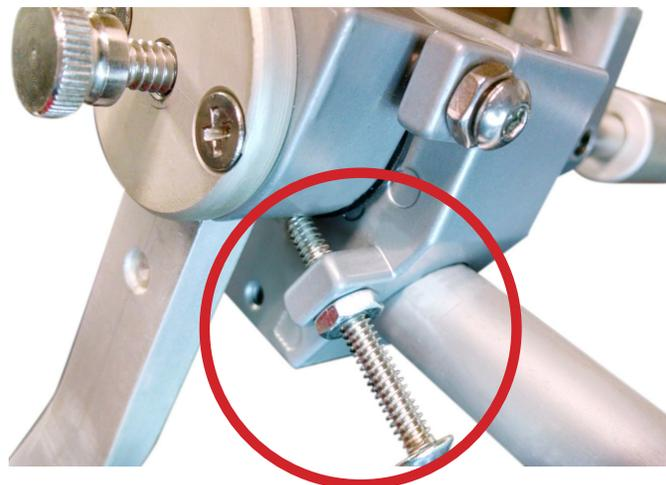
6.1. The SitGo's collapsible setting is locked when shipped from the factory. Once you have adjusted it to your pet's size and once your pet has acclimated to using a wheelchair, you can adjust or completely remove the bolt shown above to activate the SitGo's collapsible feature. Please note that the spring tension will need to be adjusted for the weight of your pet (see number 7 of this section).
