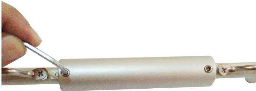
4.1. Loosen the socket set screws on the pivot shaft connector with the small hex wrench (J-2).
