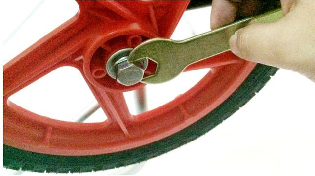
3.9. Tighten or loosen the wheel bolts with the big wrench (J-1) if necessary to ensure free-wheeling movement of the wheels.
