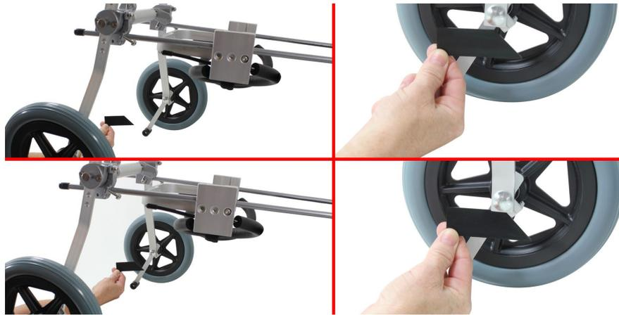
5.2. Place plastic wheel acuator alignment tool as shown in diagram to recalibrate properly.
