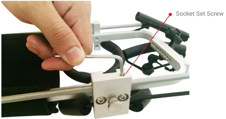
3.1. Loosen Socket Set Screws located on both sides of the Rear Harness Bars with the Hex Wrench.
