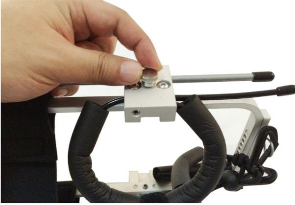
2.2. Loosen the Rear Wheel Thumb Screws.
